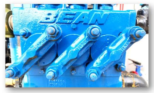
If water being pumped is corrosive or may harden when pumps are left idle, flushing of the suction lines, discharge lines, and pumps is required. Valve positions for flushing of the piping system will be dependent on fluid/media being used to flush and operator preference.
