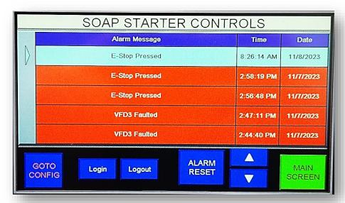
Figure 4 - Alarm Screen showing faults
