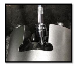
5. **ALTERNATIVELY** – USING A HOLLOW SLIDE ARM (SLIDE HAMMER), SCREW A THREADED ROD INTO THE RETENTION PIN. SCREW A NUT ON TO THE TOP END OF THE THREADED ROD AND PULL OUT THE RETENTION PIN USING THE HOLLOW SLIDE AS A REVERSE IMPACT DEVICE.
