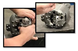
3. USING A M10-1.5 TAP, THREAD INTO THE RETENTION PIN TO CLEAN THE THREADS FOR REMOVAL.
