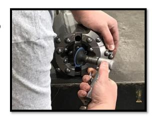
2. SLIDE THE WINGS OUT OF THE GUIDE DEVICE BY SLIDING THEM INWARD TOWARDS THE CENTER OF THE BIT. THIS PROVIDES EASIER ACCESS TO THE RETENTION PIN FOR THEIR SUBSEQUENT REMOVAL.
