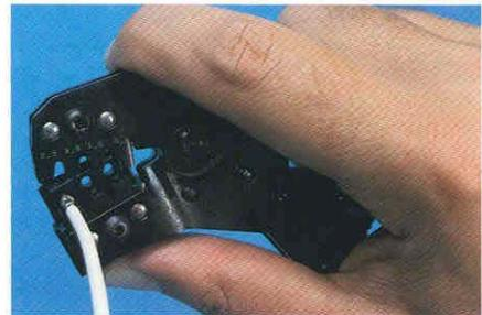
6. While pressing upward on the locator spring withdraw the crimped termination.
