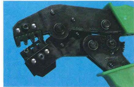
3. When correctly positioned, the contact should be located beyond flush with the edge of the hand tool and positioned on the concave polished split level crimp areas.
