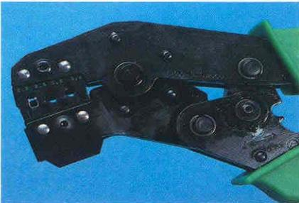
4. Partially (usually the first click) cycle the hand tool assuring that the upward thrusting tails of the contact has started engaging with the top jaw of the tool. (There is a slight tendency for the contact to roll out of vertical alignment.)
