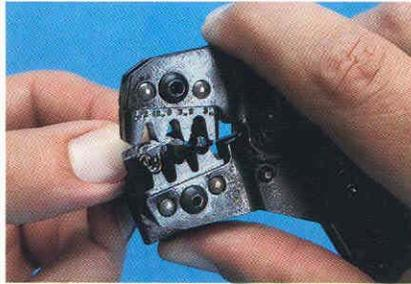
2. While pressing upward on the locator spring, insert the contact with the tails upward completely into the locator.
