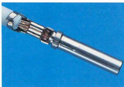
8. Note that there are no unterminated wire strands, and that some strand ends can be seen at the forward edge of the crimp. Also note the insulation is gripped by the smaller secondary crimp. Distortion is at a minimum.
