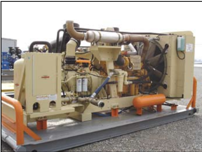
1170 CFM/350 PSI with Aftercooler Mounted on Heavy Duty Oil Field Skid
